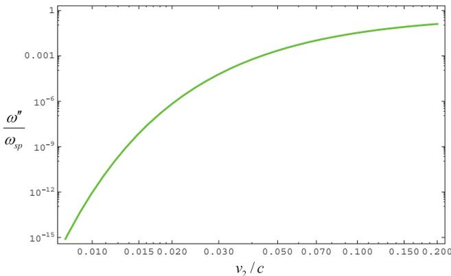
FIG. 9. (Color online) Similar to Fig. 8(b), but  $\omega''$  is calculated as a function of  $v_2$  for  $k_x = 2\omega_{sp}/v_2$ ,  $\Gamma = 0$ , and  $k_y = 0$ . The calculation is nonrelativistic and only the mode with  $\omega'' > 0$  is represented.
