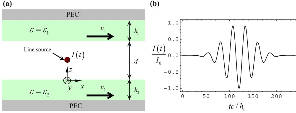
FIG. 6. (Color online) (a) A line source in between two moving dielectric slabs is excited by a current pulse. (b) The current pulse used in the numerical simulations.
