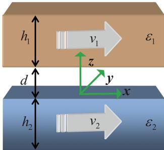
FIG. 1. (Color online) Geometry of the system: two infinitely extended (in the  $x$  and  $y$  directions) material slabs separated by an air gap with thickness  $d$  are in relative motion.
