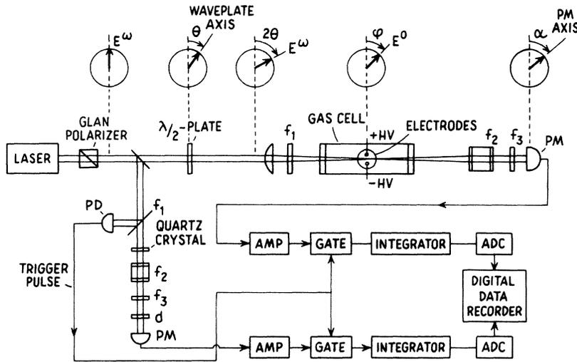
FIG. 1. Schematic diagram of the apparatus:  $d$ , diffuser;  $f_1$ , red filter;  $f_2$ , aqueous  $\text{CuSO}_4$  filter;  $f_3$ ,  $2\omega$  interference filter; PM, photomultiplier RCA type 4818; PD, photodiode RCA type 922.
