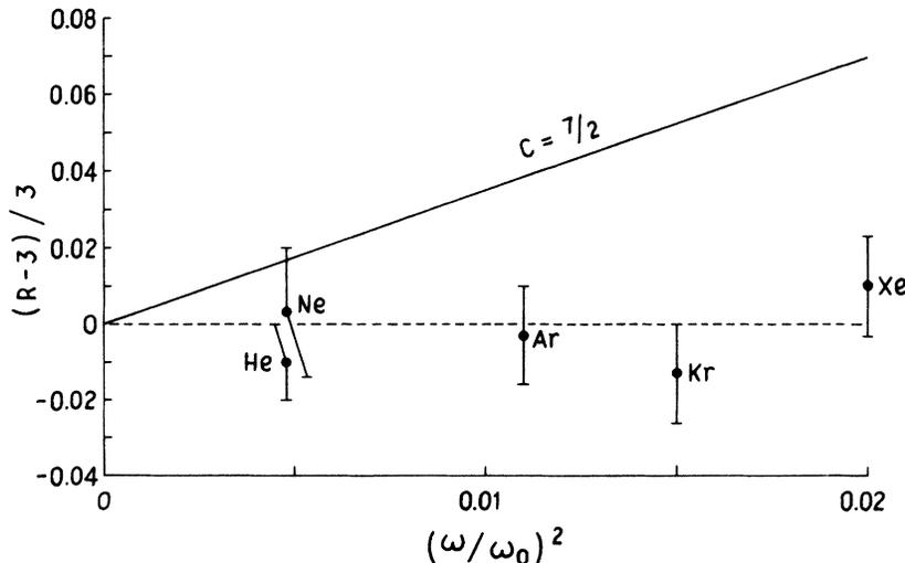
FIG. 3.  $R$  [defined in Eq. (2)] for the inert gases as a function of  $(\omega/\omega_0)^2$  where  $\omega = 0.066$  a.u. is the ruby-laser frequency and  $\omega_0$  is a characteristic frequency which varies from atom to atom. The solid line shown is predicted by Eq. (11'). Error flags on the data indicate standard deviations.
