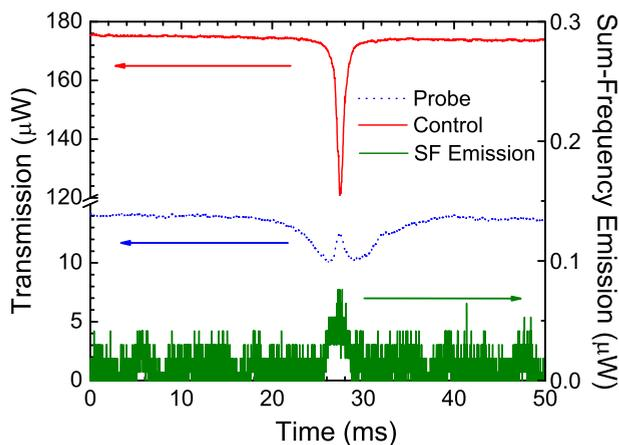
FIG. 2. (Color online) Line splitting in a quasi-CW regime: provided the phase matching, the control field coupling into the resonator suppressed the the signal field coupling; a small amount of the sum frequency is generated.
