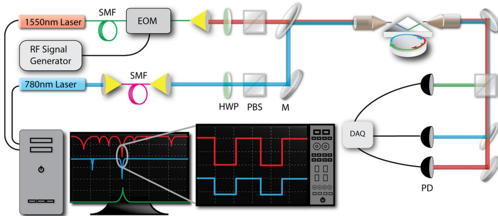
FIG. 1. (Color online) Experimental setup. PD, photodetector; M, mirror; DM, dichroic mirror; PBS, polarization beam splitter; HWP, half-wave plate; DAQ, data acquisition unit; and EOM, electro-optical modulator producing pulses. Objective lenses ( $10\times$ ) were used to focus the lasers onto the prism-resonator interface and to collect the output light.
