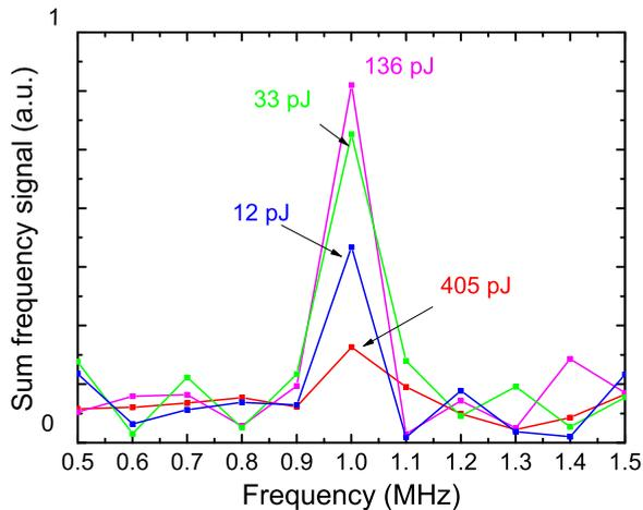
FIG. 4. (Color online) Under the coupling conditions for the interaction-free modulator, a decrease in SF efficiency was observed as the control power increased.
