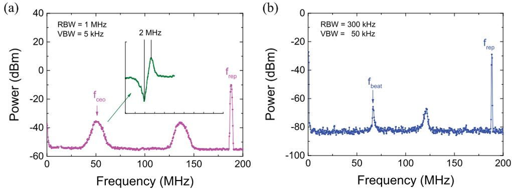
FIG. 2. (Color online) (a) Carrier-envelope offset frequency  $f_{\text{ceo}}$  of the YLFC measured using the  $f - 2f$  interferometer in Fig. 1(b) with a linewidth of 15 MHz. Inset: Frequency discriminator signal obtained with the NBF in Fig. 1(b). (b) Measured beat frequency  $f_{\text{beat}}$  between the probe laser at 1077.3 nm and the nearest comb component of the YLFC.
