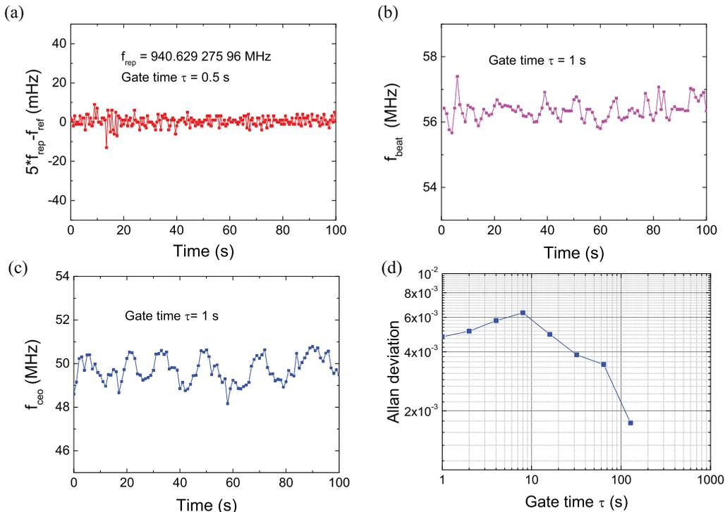
FIG. 3. (Color online) Measured (a)  $f_{\text{rep}}$ , (b)  $f_{\text{beat}}$ , and (c)  $f_{\text{ceo}}$  as a function of time. In (b), the operating current of the Yb HCL was 1.74 mA. (d) Allan deviation of  $f_{\text{ceo}}$  associate with the frequency fluctuation in (c).
