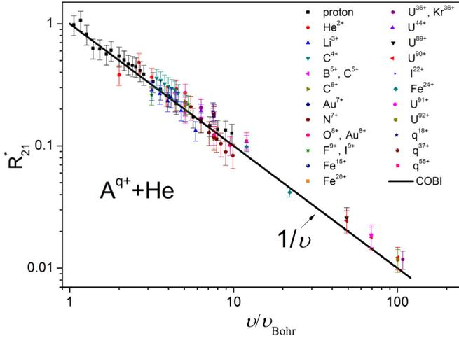
FIG. 1. (Color online) Scaled double to single ionization ratio  $R_{21}^* = R_{21}/[f(q_1, q_2) \cdot \sqrt{q_2}]$  of helium impacted by nearly stripped ions from the proton to  $U^{92+}$  ( $0.5 < q/v < 5$ ). Dots with error bars are experimental data taken from Refs. [9,11,14–19] and the line is derived from Eq. (14).
