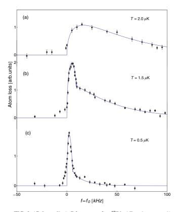
FIG. 2. (Color online) Rf spectra for <sup>87</sup>Rb  $|F = 1, m_F = -1\rangle$  atoms after evaporative cooling in the 1D magnetic lattice to trap depths  $\delta f = (f_f - f_0)$  of (a) 600 kHz, (b) 400 kHz, and (c) 100 kHz in lattice site 38. The solid lines represent fits to the data based on a self-consistent mean-field model for a BEC plus thermal cloud as described in the text.
