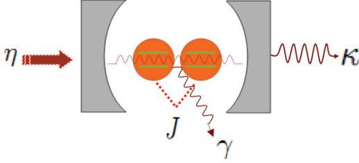
FIG. 1. (Color online) Schematic representation of two two-level atoms with dipole-dipole interaction intensity  $J$  interacting with a single-mode high-finesse cavity. The decay rates of atoms and cavity field are  $\gamma$  and  $\kappa$ , respectively. The cavity is pumped by a coherent laser field with strength  $\eta$ .
