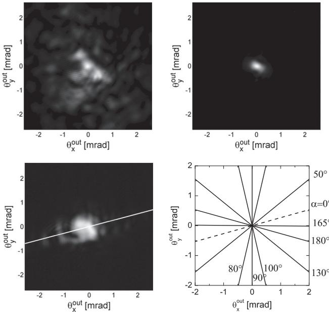
FIG. 2. Experimental angular spectra of the first (top left) and second (top right) fundamental beams as well as generated second-harmonic beam (bottom left). White line: Eq. (46). Bottom right: spectral lines for intersection planes rotated by the angle  $\alpha$  with respect to  $yz$  plane, Eq. (48).
