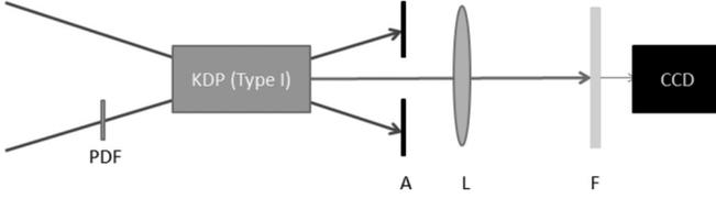
FIG. 1. Experimental setup. PDF: phase distortion film; A: aperture, L: lens; F: neutral filter.
