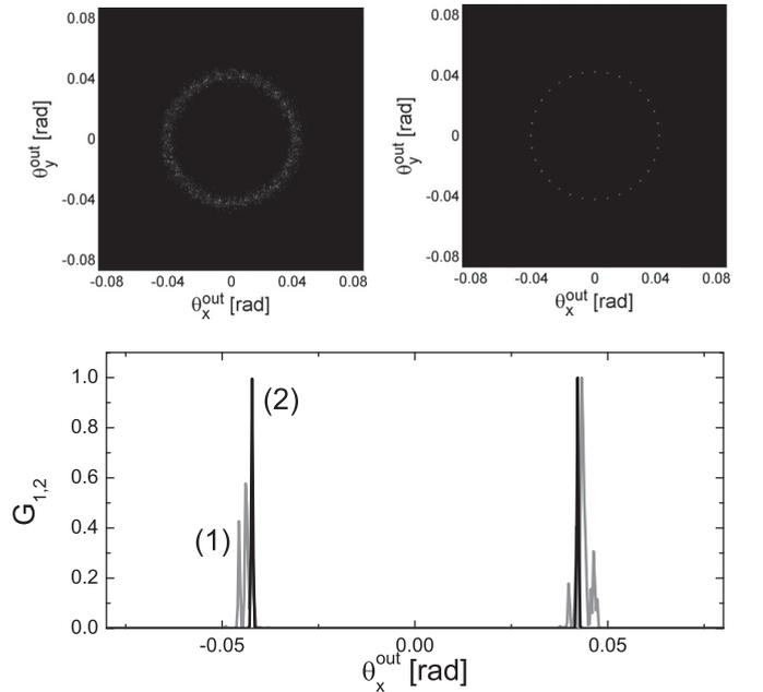
FIG. 4. Numerically calculated spectra of the first (top left) and the second (top right) fundamental beams. Bottom: normalized spectra of the first (1) and the second (2) fundamental beams at  $\theta_y^{\text{out}} = 0$ . Type-I KDP crystal, fundamental wavelength  $\lambda_1 = 1.064 \mu\text{m}$ ,  $\theta_0^{\text{out}} = 2.7^\circ$ ,  $\Delta\beta/k_0 = 2 \text{ mrad}$ ,  $d = 700 \mu\text{m}$ ,  $N = 32$ . One simulation.
