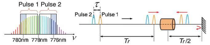
FIG. 4. (Color online) TPT excitation scheme using spectrum split pulses. Each of the pulses is split into two subpulses with  $>778$  nm and  $<778$  nm spectral components, respectively, and a time delay  $\tau$  is introduced between the first and second subpulses.
