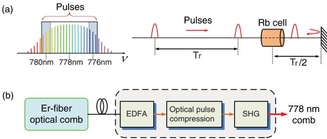
FIG. 1. (Color online) (a) Spectral components of the comb involved in the TPT excitation (left) and the regular experiment scheme (right) for TPT excitation using ultrashort pulses. (b) The optical control chain for second harmonic generation of the Er:fiber optical comb. EDFA, erbium-doped fiber amplifier; SHG, second harmonic generation.
