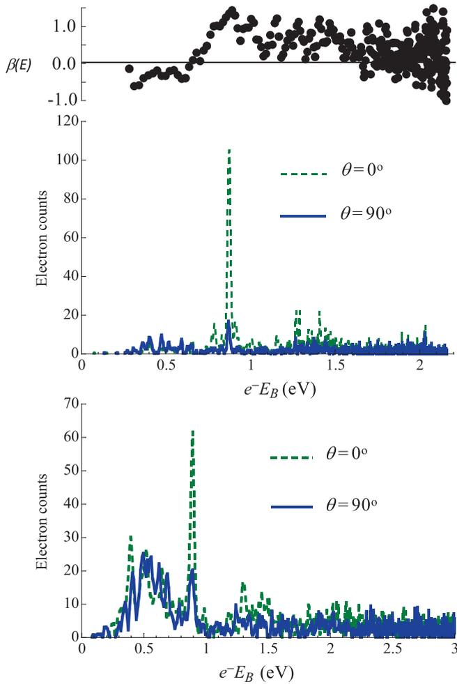
FIG. 2. (Color online) Photoelectron spectra of  $\text{Ce}^-$  obtained with the detachment laser electric field parallel to ( $\theta = 0^\circ$ , dashed green traces) and perpendicular to ( $\theta = 90^\circ$ , solid blue traces) the detected electron trajectory. Top panel spectra were collected with 2.33-eV photon energy, bottom panel spectra were collected with 3.49-eV photon energy. The asymmetry parameter determined for the 2.33-eV spectrum is shown just above the 2.33-eV spectrum.
