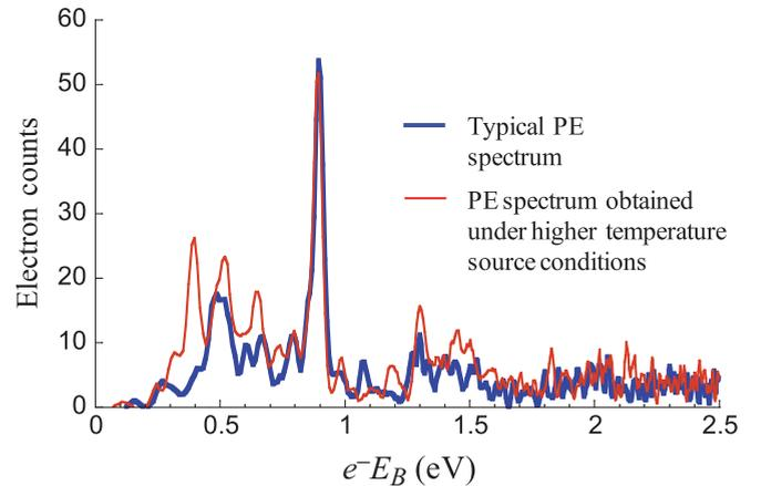
FIG. 4. (Color online) PE spectra of  $\text{Ce}^-$  obtained under different source conditions. 3.49-eV photon energy was used to collect the data.
