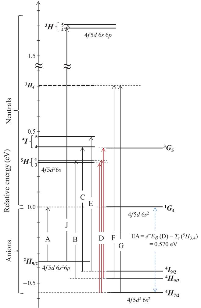
FIG. 3. (Color online) Simplified energy level diagram summarizing the relative energies of the various anion(Refs. [1,2], and this work) and neutral states (Ref. [5]) associated with the detachment transitions labeled in Fig. 1. Leading electronic configurations and LS terms are included, but note that most states are heavily mixed. The groups of transitions labeled H and I in Fig. 1 involve heavily mixed groups of final states.
