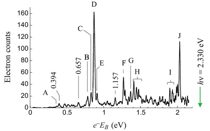
FIG. 1. (Color online) Photoelectron spectrum of  $\text{Ce}^-$  obtained using 2.33-eV photon energy, in which electrons are binned into 0.002-eV energy intervals. Peak positions and assignments for peaks labeled with letters are included in Table I. Several unassigned peaks are labeled by their position (eV) for reference.
