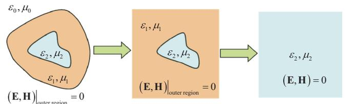
FIG. 5. (Color online) Sketch of the proof that a bounded layered structure formed by conventional isotropic materials with  $\varepsilon \neq 0$  and  $\mu \neq 0$  standing in a vacuum cannot support localized oscillations with infinite lifetimes.
