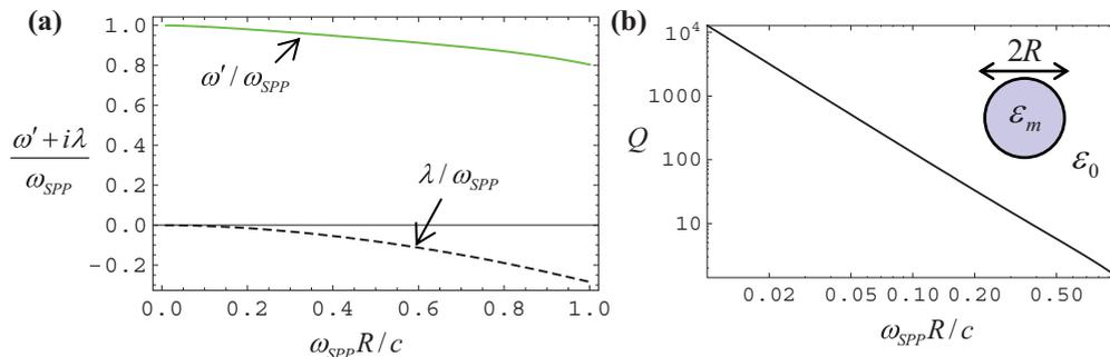
FIG. 6. (Color online) (a) Characteristic (complex) oscillation frequency of the surface plasmon supported by a cylindrical nanoparticle as a function of the normalized radius  $R$ . (b) Quality factor as a function of the normalized radius  $R$ .
