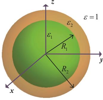
FIG. 1. (Color online) Geometry of the open bounded resonator formed by a core-shell nanoparticle. The cover shell is made of a low-permittivity (ENZ) material.
