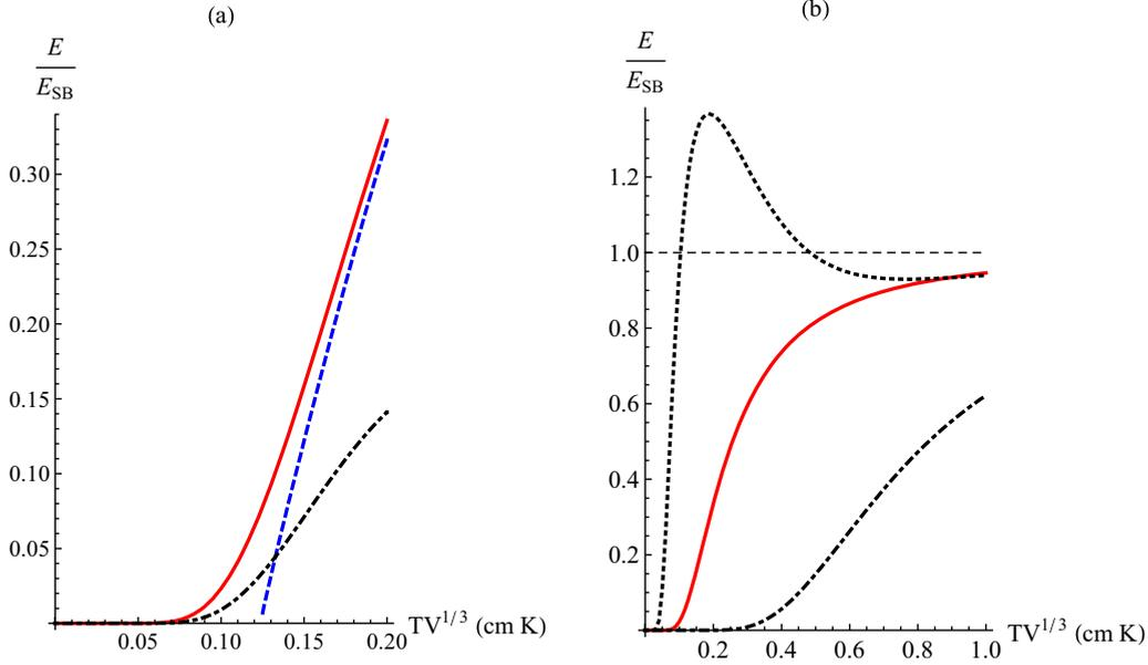
FIG. 1. (Color online) Radiation energy in a cavity normalized to the value predicted by the Stefan-Boltzmann law. (a) Cubic cavity: solid, dashed, and dash-dotted curves correspond to calculated results, high-temperature expansion [9], and low-temperature expansion [9], respectively. (b) Cuboid cavities of different shapes: solid, dotted, and dash-dotted curves correspond to  $\alpha = \beta = 1$  (cube),  $\alpha = \beta = 10$  (film), and  $\alpha = \beta = 10^{-2}$  (rod), respectively.
