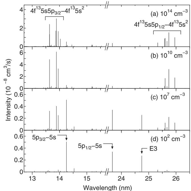
FIG. 3. Same as Fig. 1(b) but for electron densities of (a)  $10^{14}$ , (b)  $10^{10}$ , (c)  $10^7$ , and (d)  $10^2 \text{ cm}^{-3}$ .
