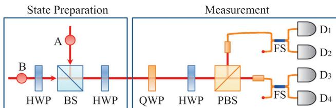
FIG. 2. (Color online) Experimental setup. Single photons A and B, both horizontally polarized, are prepared by spontaneous parametric down-conversion. (PBS denotes a (polarization) beam splitter. HWP and QWP denote half-wave and quarter-wave plates, respectively. FS denotes a 50:50 fiber splitter, and D1–D4 denote single-photon avalanche photodiodes.
