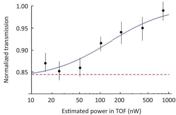
FIG. 5. (Color online) Measured TOF transmission as a function of increasing power passing through the TOF. The data points are best fit to a simple nonlinear transmission model (blue line) with an ultralow saturation power of  $(126 \pm 44)$  nW. For comparison, the dashed red line shows what would be expected from ordinary linear transmission.
