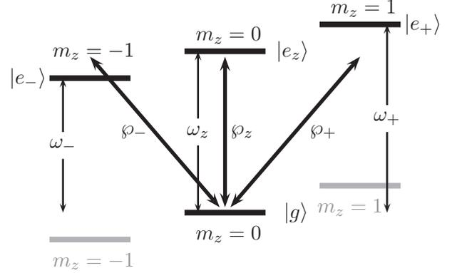
FIG. 20. Atomic level structure. We consider three excited states  $|e_\pm\rangle$  and  $|e_z\rangle$  with the frequencies  $\omega_\pm$  and  $\omega_z$ , respectively, and one ground state  $|g\rangle$ . The dipole moments  $\wp_\pm$  and  $\wp_z$  initiate transitions between sublevels and correspond to the polarizations  $\boldsymbol{\sigma}'_\pm$  and  $\boldsymbol{\sigma}'_z$  in the primed frame.
