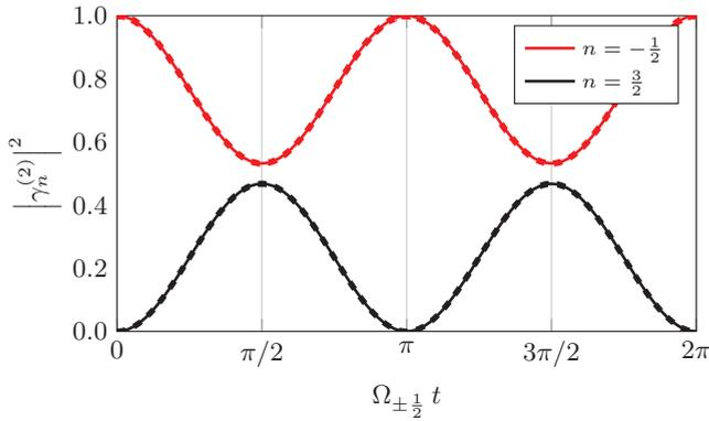
FIG. 18. (Color online) Rabi oscillations between the quasiresonances  $|\hbar K/2\rangle \leftrightarrow |3\hbar K/2\rangle$  for  $\Delta\omega = \omega_r$  (solid lines). The oscillations are suppressed by approximately one half. The dashed lines show a numerical solution of the Rabi equations for  $\varepsilon = 0.01$  and confirm our analytical result.
