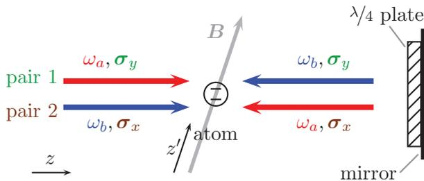
FIG. 19. (Color online) Linear-linear configuration for double Bragg diffraction. The magnetic field  $\mathbf{B}$  is not in the  $z$  direction of the pair of light fields, but in a different one denoted by  $z'$ . The polarizations of the two pairs are linear and orthogonal to the  $z$  direction of propagation, i.e.,  $\boldsymbol{\sigma}_x$  and  $\boldsymbol{\sigma}_y$ .
