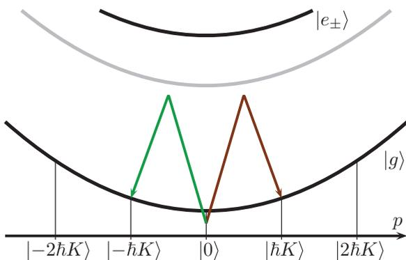
FIG. 14. (Color online) Scattering process between the states  $|\pm \hbar K\rangle$  according to Eq. (37). If the atoms are initially in one of these states, a resonant Rabi oscillation between them takes place in second-order Bragg diffraction. This phenomenon can be explained by the resonant four-photon process shown above. The transitions for other initial conditions are shown in Fig. 13.
