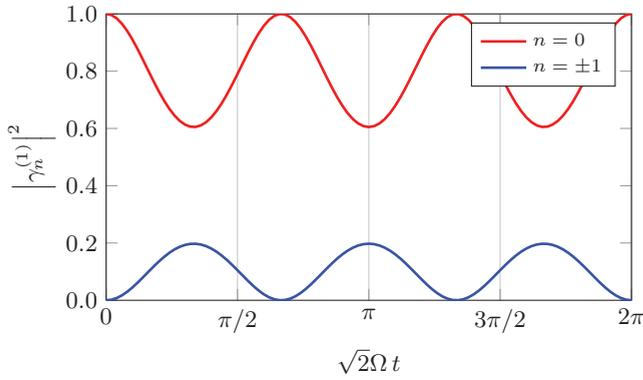
FIG. 10. (Color online) Rabi oscillations of the populations  $|\gamma_n^{(1)}|^2$  of the momentum states  $|(n + 0.01)\hbar K\rangle$  in the deep Bragg regime ( $\varepsilon = 0.01$ ) for the off-resonant momentum  $p = 0.01\hbar K$ . The Rabi oscillations are detuned and suppressed, which leads to velocity selectivity. The initial condition is  $(0, 1, 0)^T$  and the time is in units of the resonant frequency  $\sqrt{2}\Omega$ .
