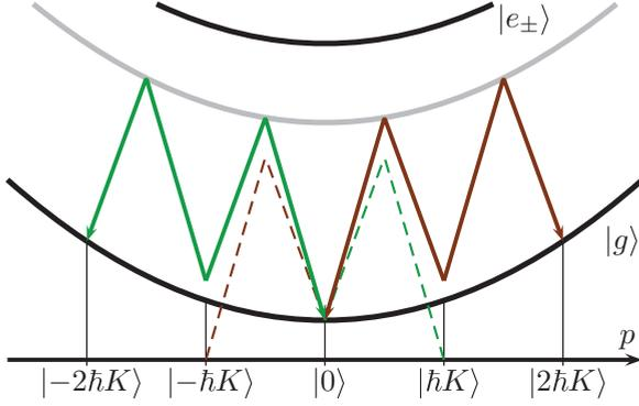
FIG. 13. (Color online) Two processes in second-order double Bragg diffraction ( $\Delta\omega = 2\omega_r$ ). A four-photon transition in each direction occurs. For an initial population of the momentum states  $|0\rangle$  and  $|\pm 2\hbar K\rangle$ , the states  $|\pm \hbar K\rangle$  are just virtually occupied. Different initial conditions are sketched in Fig. 14. The dashed lines show off-resonant processes.
