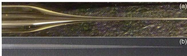
FIG. 1. (Color online) Pictures of the capillaries used in the experiment: (a) funnel-shaped capillary and (b) conical capillary.
