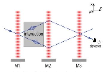
FIG. 4. (Color online) Schematic top view of our atom interferometer: the HMW interaction region is placed just before the second laser standing wave, at the place where the arm separation is largest. It is thus possible to introduce a septum between the two interferometer arms without any perturbation of the interferometer signal.
