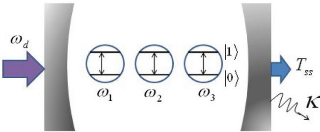
FIG. 1. (Color online) Schematics of three TLAs (with transition frequency  $\omega_1, \omega_2, \omega_3$ , respectively) dispersively coupled to a cavity. An external driving with the frequency  $\omega_d$  is applied to the cavity.  $\kappa$  denotes the cavity decay rate. The joint measurements of three TLAs can be realized by probing the steady-state transmission spectra  $T_{ss}$  of the driven cavity.
