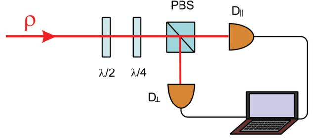
FIG. 1. (Color online) The setup for polarization tomography [10,13]. PBS is the polarizing beam splitter;  $D_{\parallel}$  and  $D_{\perp}$  are the photodetectors. The signals from the detectors are processed by either digital or analog electronics, after which a computer calculates the probability distributions  $W_{\theta\phi}(n)$  and performs the Radon transformation.
