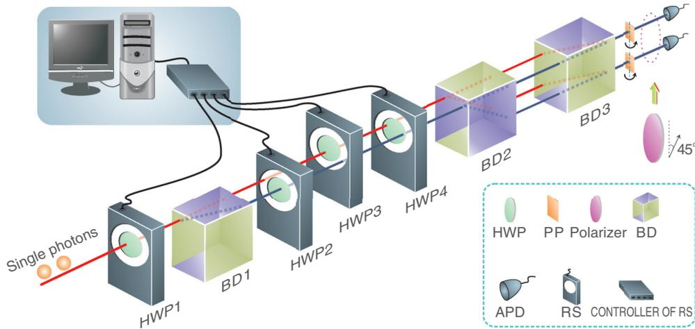
FIG. 1. (Color online) Experimental setup, showing the three stages of the experiment. Note that the parameters  $\gamma$ ,  $\theta_1$ ,  $\theta_2$ , and  $\varphi_M$  in the main text were set to variable values by modulating HWP1–HWP4, respectively, which were installed in four motorized rotation stages (RS) and computer controlled.
