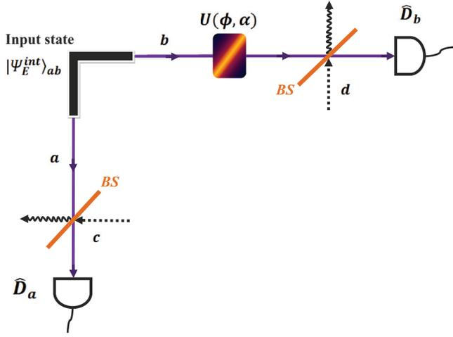
FIG. 1. (Color online) Interferometric phase estimation scheme for the entangled SU(1,1) CSs. Channel  $b$  acquires a phase  $\phi$  relative to channel  $a$ . After applying a phase shift  $\hat{U}(\phi, \alpha)$  in mode  $b$ , the parity measurement is performed.
