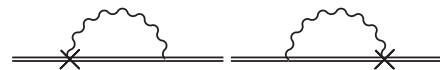
FIG. 3. The NRQED diagrams for the self-energy with modified vertex interactions at order m\alpha^7 .
