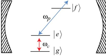
FIG. 1. (Color online) Interaction scheme of a  $\Xi$ -type three-level atom in a cavity. The atomic states  $|g\rangle$  and  $|e\rangle$  and a cavity field mode of frequency  $\omega_c$  form a quantum Rabi model described by  $H_R$ , and an external classical field of frequency  $\omega_p$  drives the transition between  $|e\rangle$  and  $|f\rangle$ .
