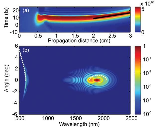
FIG. 3. (Color online) (a) Computed pulse temporal evolution during filamentation in a 3-cm-long fused silica sample. The input pulse has central wavelength  $\lambda_0 = 1.9 \mu\text{m}$ , duration 70 fs, and energy 7.2  $\mu\text{J}$ . The black line marks the slope for calculating the velocity of the intensity peak. (b)  $(\theta, \lambda)$  spectrum obtained by numerical simulation. The dashed curves show the fit with Eq. (2).
