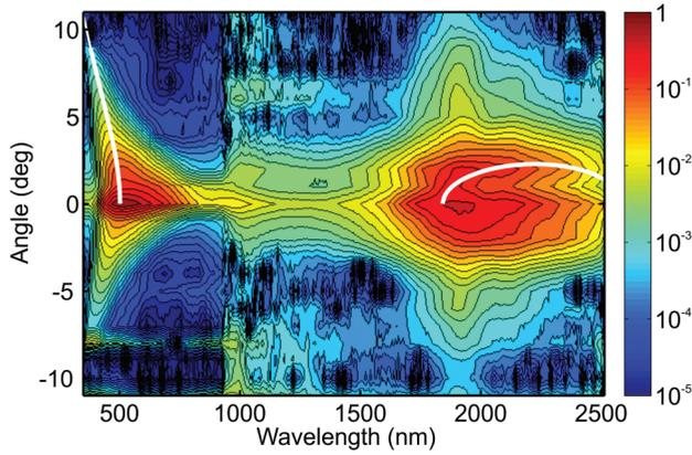
FIG. 4. (Color online) Angular distribution of the conical emission, after filamentation of 1.9- $\mu\text{m}$ , 40-fs, 26- $\mu\text{J}$  pulses in 3 cm of fused silica. This figure has a logarithmic scale. The white curves show the fit with Eq. (2).
