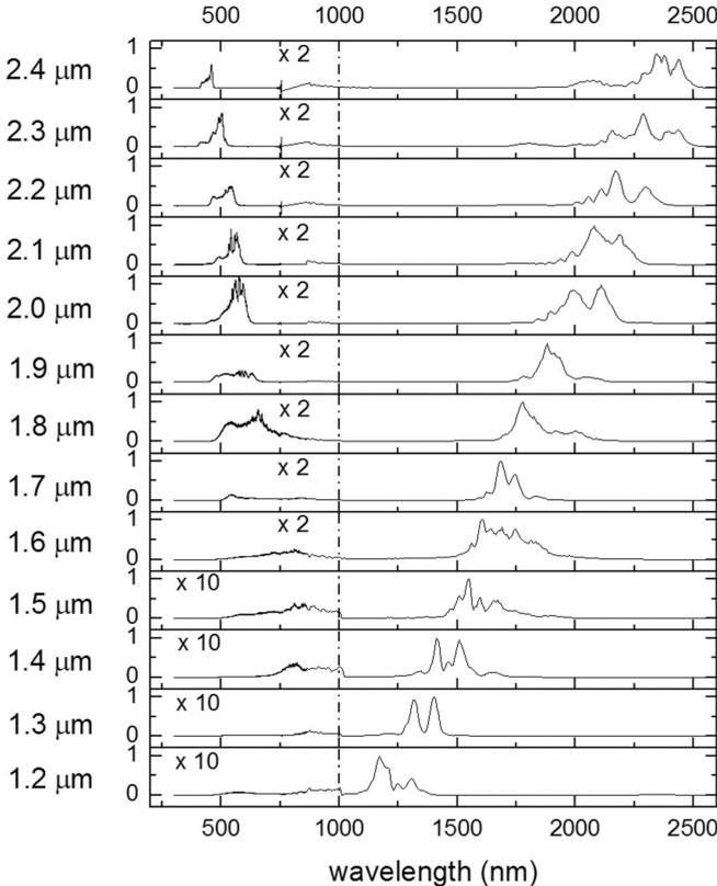
FIG. 2. Spectra measured at the center of the conical emission after filamentation in a 4-cm-thick fused silica sample. The central wavelength used for filamentation ranged from 1.2 to 2.4  $\mu\text{m}$ . The visible part of the spectra up to 1  $\mu\text{m}$  is magnified by a factor of 10 for  $\lambda_0$  (1.2–1.5  $\mu\text{m}$ ) and by a factor of 2 for  $\lambda_0$  (1.6–2.4  $\mu\text{m}$ ).
