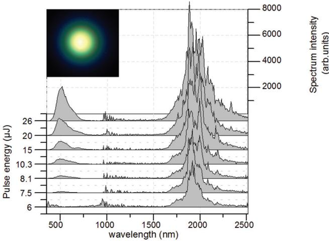
FIG. 1. (Color online) Supercontinuum measured at the center of the conical emission after filamentation in 3 cm of fused silica of a 1.9- $\mu\text{m}$ , 35-fs pulse at different input energies. Inset: Photo of the conical emission at 15  $\mu\text{J}$ .
