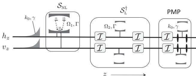
FIG. 5. The cascadable primitive gate. First, nonlinear evolution is provided by interaction with the atomic  $\vee$  system. Linear evolution is then removed. Finally, principal-mode projection is performed.
