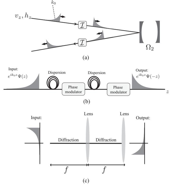
FIG. 2. (a) Optical circuit to simulate time-reversed evolution under Eq. (14). The cavity frequency  $\Omega_2$  is chosen so that  $k_0 - \Omega_1 = -(k_0 - \Omega_2)$ . (b) Temporal imaging system to realize inversion  $\mathcal{I}$  about center frequency  $k_0$ , using two dispersive delay lines and two quadratic phase modulators. (c) The analogous spatial imaging system using free-space diffraction and thin lenses.
