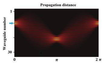
FIG. 6. (Color online) Wave packet dynamics: evolution of a discrete Gaussian beam in a  $J_x$  waveguide array. The blue arrow indicates the waveguide where the wave packet is initially centered.
