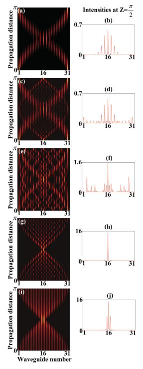
FIG. 7. (Color online) Left column depicts the calculated intensity propagation when light is launched into (a) the first and 31st sites, (c) the first, 16th, and 31st sites, (e) the first, fifth, tenth, 16th, 22nd, 27th, and 31st sites, (g) every other site (n = odd), and (i) every site. In all the cases we have considered unitary input intensities at every excited waveguide. Right column shows the intensity distributions at  $Z = \frac{\pi}{2}$  for each case.
