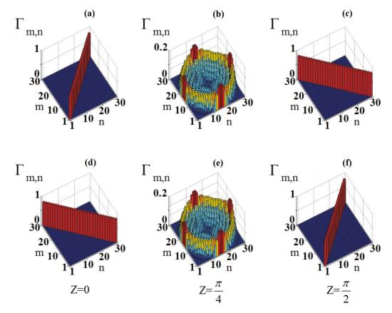
FIG. 4. (Color online) (a)–(c) Upper row shows the calculated quantum correlation maps when the correlated input state  $|\psi_C\rangle$  is coupled into a  $J_x$  photonic lattice. (d)–(f) Similarly, bottom row depicts the correlation evolution for the anticorrelated input state  $|\psi_A\rangle$ .
