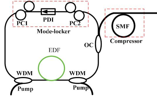
FIG. 1. (Color online) Experimental configuration of the laser.
