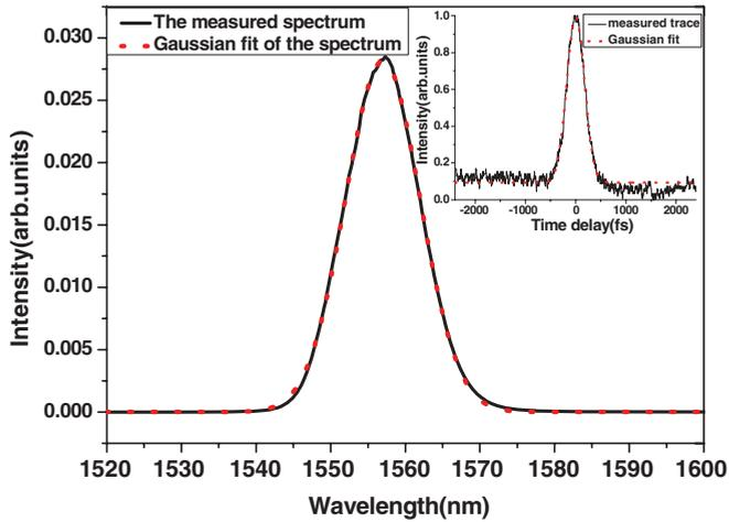
FIG. 2. (Color online) The spectrum and autocorrelation trace (inset) of the DM solitons (solid black line) and the Gaussian fit (dotted red line).
