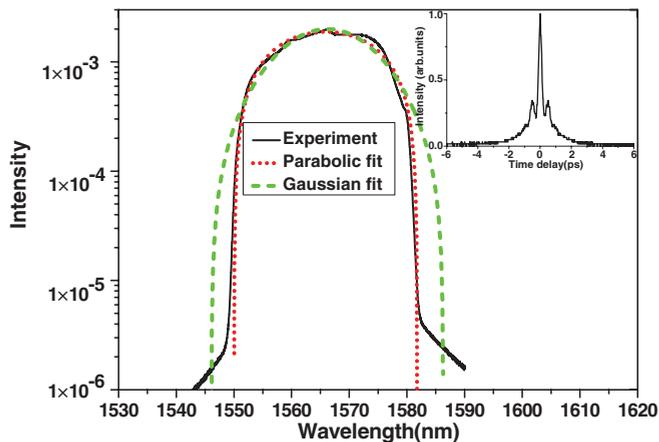
FIG. 7. (Color online) The measured spectrum of similaritons (solid black line), and Gaussian (dashed green line) and parabolic (dotted red line) fits. The inset shows the autocorrelation trace.
