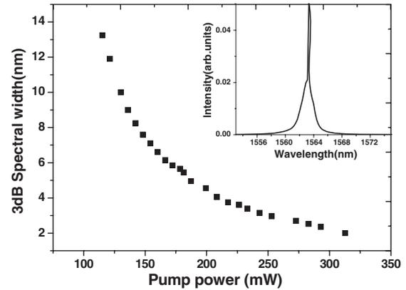
FIG. 4. The spectral width scaling with pump power and the spectrum of the cw (inset).
