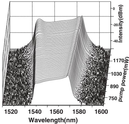
FIG. 6. Pulse spectrum of DS scaling with pump power.
