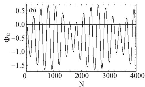
FIG. 4. (a) Simulated  $x$ - $y$  trajectory of a particle as it moves  $N = 4000$  twists = 100 m through the helical guide described in the text. (b) Accumulated geometric phase after a particle with the initial conditions described in the text travels from a uniform field region, through a helical guide of  $N$  turns, and exits into a second region of uniform field region.
