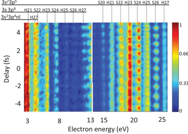
FIG. 3. (Color online) Electron spectrum as a function of time delay between the attosecond pulses and the IR laser. The signal strength is indicated by colors. The spectrum on the right ( $3p$ ) follows that on the left ( $3s$ ) with a factor of 6 reduction in the color code and a slight overlap in energy.
