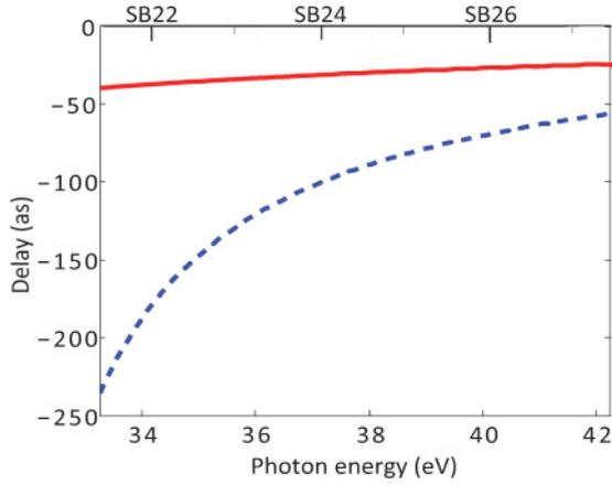
FIG. 5. (Color online) Continuum-continuum delay  $\tau_{cc}$  as a function of excitation photon energy for subshells  $3s$  (red solid line) and  $3p$  (blue dashed line) for an IR photon energy of 1.55 eV (800-nm wavelength).
