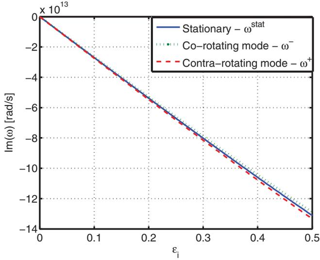
FIG. 2. (Color online) The imaginary part of the resonant frequencies of a lossy ring resonator when stationary and when rotating.
