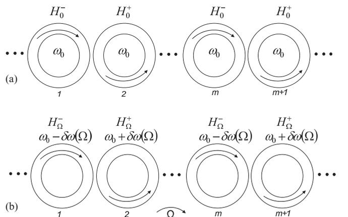
FIG. 5. CROW consisting of doubly degenerate ring resonators: (a) stationary, (b) rotating.
