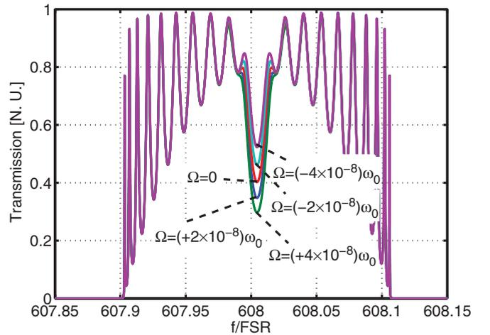
FIG. 8. (Color online) Transmission (normalized units) of a “biased” CROW as a function of frequency (normalized to the free spectral range of a single resonator with  $\omega_0$ ) for various rotation rates.
