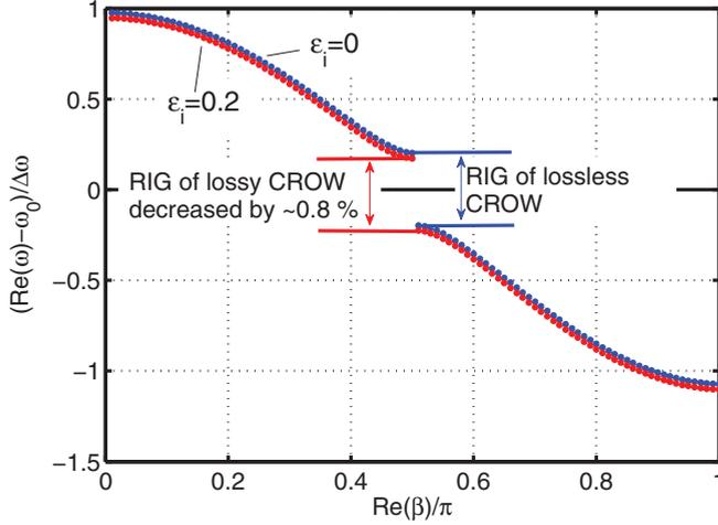
FIG. 6. (Color online) Transmission function of the rotating lossless and lossy CROWs.
