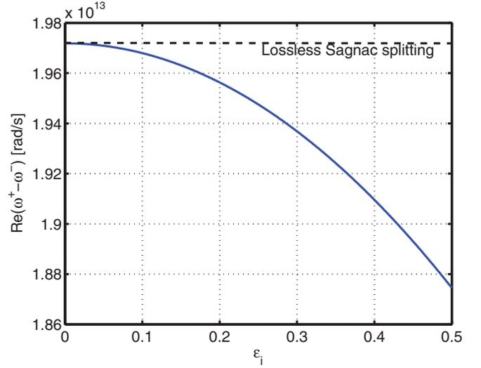
FIG. 4. (Color online) Sagnac frequency splitting of a ring resonator, as a function of the imaginary part of relative permittivity. The dashed line shows the value for a lossless resonator.
