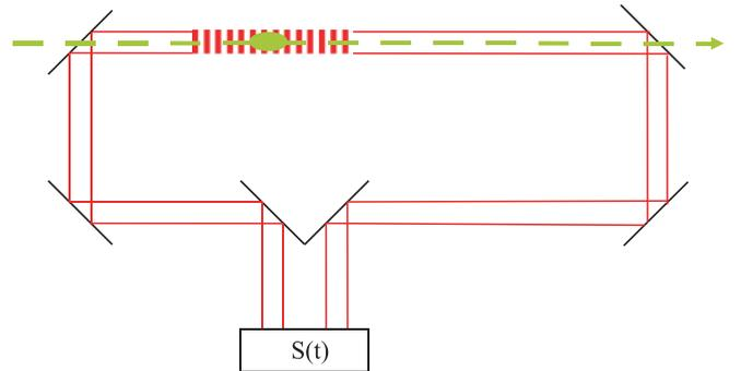
FIG. 2. (Color online) Scheme of the comoving optical potential slower. A far-off-resonance, linearly polarized standing wave ( $\lambda = 811.5$  nm) is produced by a separated-arm interferometer. Light intensity is modulated in time by a signal  $S(t)$  (see text). The atom beam is introduced with a small inclination through holes drilled in the mirrors.
