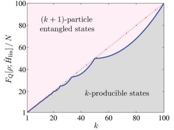
FIG. 1. (Color online)  $F_Q^{k+1}$  criterion. The solid line is the bound  $F_Q[\rho; \hat{H}_{\text{lin}}] = sk^2 + r^2$  which separates  $k$ -producible states (below the line) from  $(k+1)$ -particle entangled states (above the line). For comparison, the function  $F_Q[\rho; \hat{H}_{\text{lin}}] = Nk$  is plotted (dotted line). Here  $N = 100$ .
