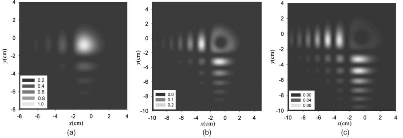
FIG. 1. Intensity distribution of the Airy beam at the initial plane (a) without an obstacle, (b) for  $b_x = b_y = -0.6$  cm and  $w_0 = 1.5$  cm, and (c) for  $b_x = b_y = -0.5$  cm and  $w_0 = 3$  cm.
