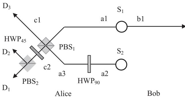
FIG. 1. Schematic of the single-photon-assisted ECPs with linear optics.  $S_1$  is the partial entanglement source and  $S_2$  is the single-photon source. PBSs transmit the horizontal polarization component and reflect the vertical component. HWP<sub>90</sub> and HWP<sub>45</sub> rotate the polarization of the state by 90° and 45°, respectively.
