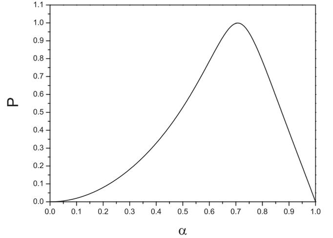
FIG. 4. Success probability  $P$  of getting a maximally entangled state after performing the QND2 protocol ( $N \rightarrow \infty$ ) is altered with the entanglement of the initial partially entangled state (i.e.,  $\alpha$ ). For the numerical simulation, we chose  $N = 10$  as a good approximation.
