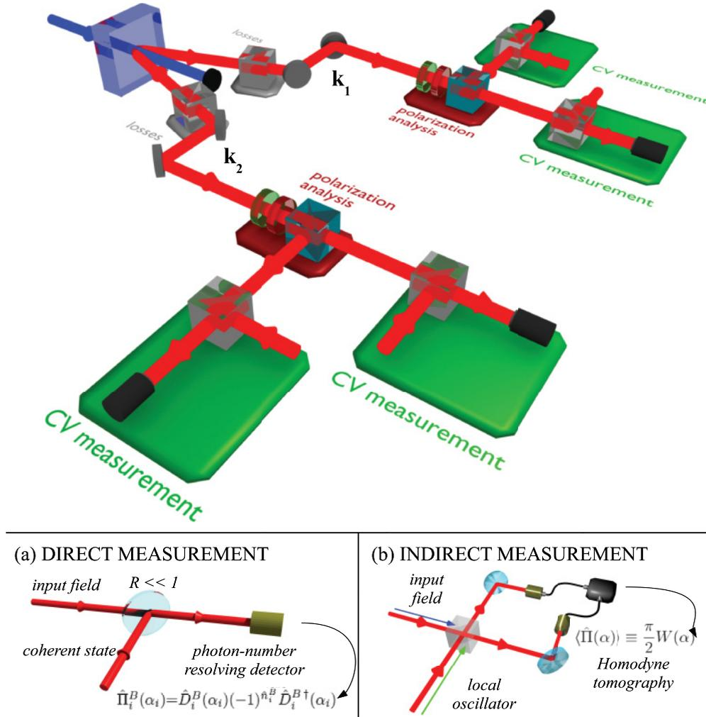
FIG. 1. (Color online) Scheme of the multiphoton source and of the detection apparatuses for the measurement of the continuous-variable Bell's test. The two spatial modes are split according to polarization, resulting in four modes which can be analyzed with independent detection systems. Losses are modeled by an additional beam-splitter. (a)–(b) Apparatuses for the direct (a) and indirect (b) measurement of the displaced parity operators.
