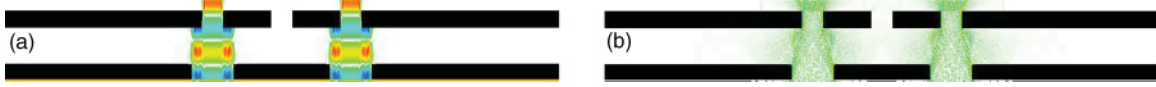
FIG. 4. (Color online) Two-dimensional representation of the experiment reported in Ref. [2]. The three slits at the top are 30 \mu\text{m} wide, their centers being separated by 100 \mu\text{m} . The blocking mask at the bottom can have one, two, or three slits, each slit being 60 \mu\text{m} wide with its center aligned with one of the slits in the top plate [2]. In the example shown, the middle slit of the blocking mask is closed (corresponding to the case OCO ). The separation between the top plate and blocking mask is 50 \mu\text{m} . The index of refraction of the 25\text{-}\mu\text{m} -thick material (colored black) is 2.29 + 2.61i (index of refraction of steel at 405 \text{ nm} ). The wavelength of the incident light is 405 \text{ nm} . Also shown are the amplitudes of the (a) E_x and (b) E_z components of the electric fields as obtained from a FDTD solution of Maxwell's equation for a monochromatic light source (not shown) illuminating the blocking mask. Note that the E_x and E_z components propagate in a very different manner.
