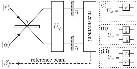
FIG. 1. An interferometric scheme with coherent and squeezed vacuum states interfered at a beam-splitter, with arbitrary quantum measurement potentially involving an additional reference beam. In general, the QFI bounds on the phase-estimation precision depend on the way the interferometer phase delay is modeled: (i) phase shift only in the upper arm, (ii) phase shift distributed symmetrically, (iii) phase shifts defined with respect to an additional reference beam.
