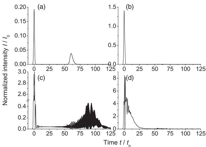
FIG. 4. Shape of the reflected intensity at different peak amplitudes of the incident pulse: (a)  $A_m = A_0$ , (b)  $A_m = 3A_0$ , (c)  $A_m = 5A_0$ , and (d)  $A_m = 7A_0$ . The central wavelength of the pulse spectrum is  $\lambda_c = 1.064 \mu\text{m}$ .
