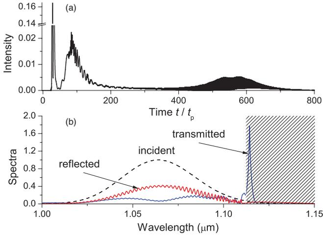
FIG. 6. (Color online) (a) Shape of the transmitted intensity. (b) Spectra of reflected and transmitted radiation. The peak amplitude of the incident pulse is  $A_m = 3A_0$ . Calculations were performed for a photonic crystal with linear  $A$  layers (first layers of the period). The band gap of the linear photonic crystal is shaded.
