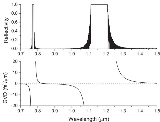
FIG. 2. Spectral curves for reflectivity (upper panel) and group velocity dispersion (lower panel) of the photonic crystal under consideration. The parameters of the structure are given in the text.
