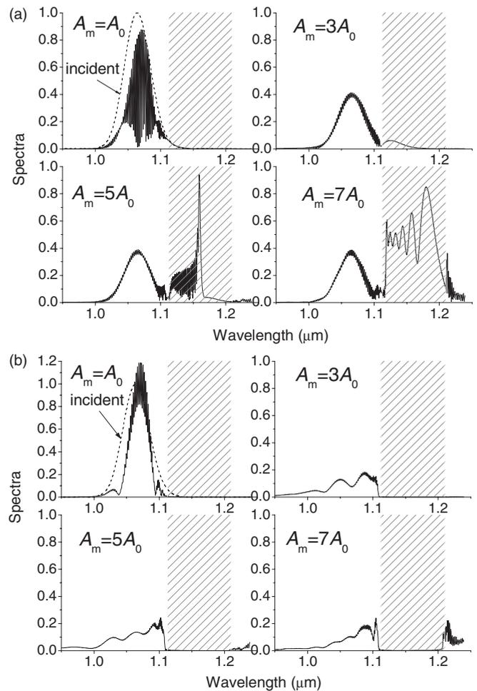
FIG. 5. Spectra of (a) reflected and (b) transmitted radiation at different peak amplitudes  $A_m$  of the incident pulse corresponding to those used in Fig. 4. The dashed curve depicts the spectrum of the incident Gaussian pulse. The band gap of the linear photonic crystal is shaded.
