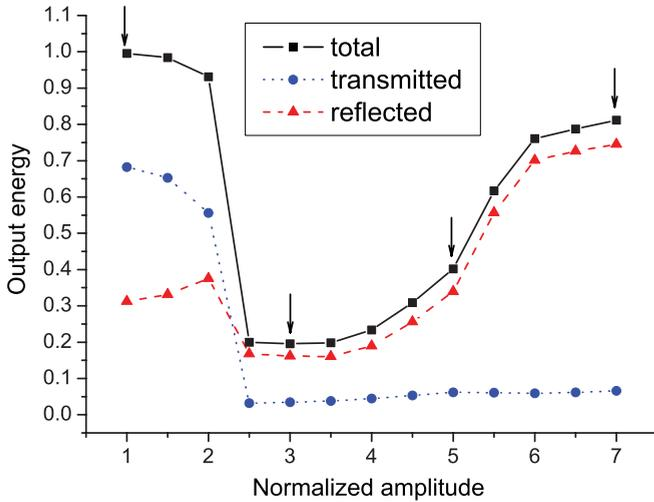
FIG. 1. (Color online) Dependence of the output light energy (normalized to the input energy) on the peak amplitude of the incident pulse. Energy is integrated over the time  $200t_p$  (about six times larger than the pulse transmittance time in the linear regime).
