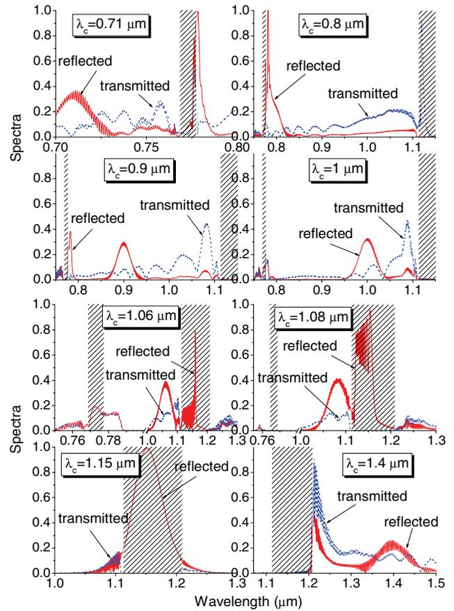
FIG. 7. (Color online) Spectra of reflected and transmitted radiation at different central wavelengths  $\lambda_c$ . The peak amplitude of the incident pulse is  $A_m = 5A_0$ . The band gap of the linear photonic crystal is shaded. The position of the spectrum of the incident pulse is characterized by the bell-shaped curve in the spectrum of the reflected light.
