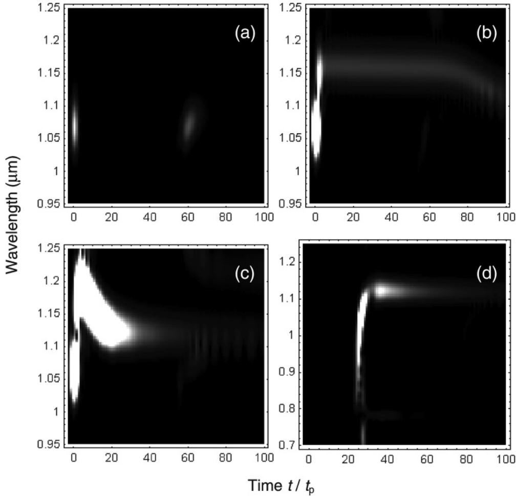
FIG. 8. (a)–(c) Spectrograms of reflected radiation at peak amplitudes of the incident pulse  $A_m = A_0$ ,  $5A_0$ , and  $7A_0$ , respectively. The central wavelength is  $\lambda_c = 1.064 \mu\text{m}$ . (d) Spectrogram of transmitted radiation at  $A_m = 5A_0$  and  $\lambda_c = 0.8 \mu\text{m}$ .
