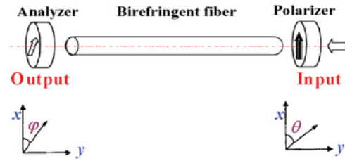
FIG. 7. (Color online) An equivalent setup to NPR element for determining the cavity transmission.
