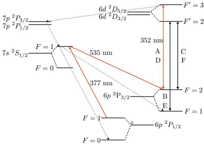
FIG. 1. (Color online) Energy levels of a Tl atom, showing the ground state and the first few excited states. The “A”, “B”, and “C” hyperfine transition lines are for  $^{205}\text{Tl}$ . The “D”, “E”, and “F” hyperfine transition lines are for  $^{203}\text{Tl}$ .
