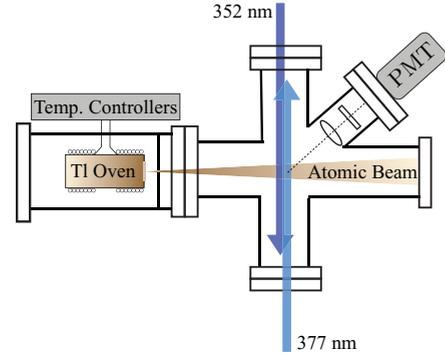
FIG. 2. (Color online) Schematic of the main chamber where the counterpropagating optical pumping (377 nm) and cooling laser beams (352 nm) intersect with the collimated Tl atomic beam. A photomultiplier tube (PMT) is used to collect the fluorescence signal.
