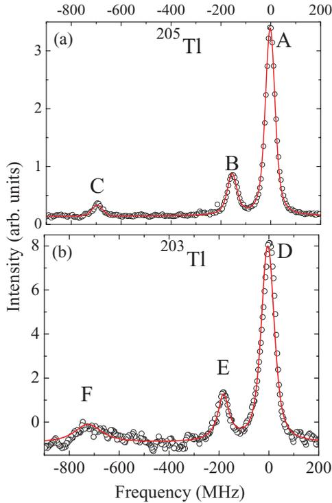
FIG. 5. (Color online) The  $6P_{3/2} \leftrightarrow 6D_{5/2}$  hyperfine spectra of (a)  $^{205}\text{Tl}$ , with A ( $F = 2 \rightarrow F' = 3$ ), B ( $F = 1 \rightarrow F' = 2$ ), and C ( $F = 2 \rightarrow F' = 2$ ) lines, and (b)  $^{203}\text{Tl}$  with D ( $F = 2 \rightarrow F' = 3$ ), E ( $F = 1 \rightarrow F' = 2$ ), and F ( $F = 2 \rightarrow F' = 2$ ) lines. Solid lines are the fits; circles are the data points.
