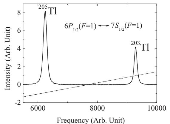
FIG. 4. Optical pumping transition for the two isotopes. The straight line represents the frequency ramping signal of the laser. The PMT was biased at 0.7 kV and the lock-in amplifier settings were as follows: 10-mV sensitivity,  $T_c = 10$  ms/12 dB,  $\theta = 159.98^\circ$ , and  $f_{\text{ref}} = 2$  kHz. The oven pressure (450 °C) was  $4.1 \times 10^{-7}$  Torr.
