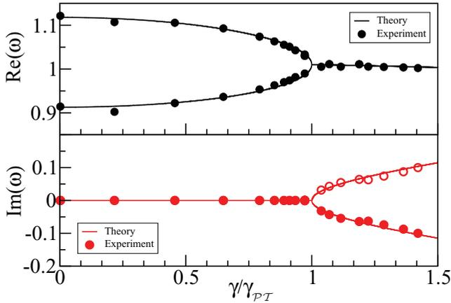
FIG. 2. (Color online) Parametric evolution of the experimentally measured eigenfrequencies vs the normalized gain and loss parameter  $\gamma/\gamma_{\mathcal{PT}}$ . A comparison with the theoretical results of Eq. (4) indicate an excellent agreement. In all cases, we show only the  $\text{Re}(\omega) > 0$  eigenfrequencies. The open circles in the lower panel are reflections of the experimental data (lower curve) with respect to the  $\text{Im}(\omega) = 0$  axis.
