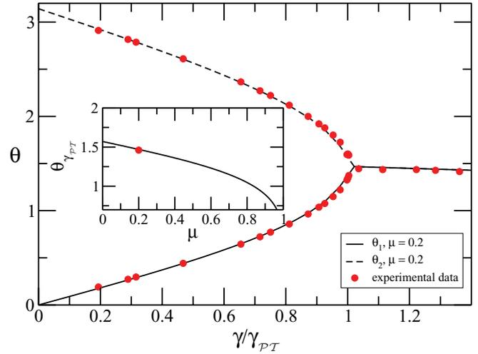
FIG. 3. (Color online) Parametric evolution of the phase difference  $\theta_l = \phi_2^{(l)} - \phi_1^{(l)}$ . The experimental measurements for  $\mu = 0.2$  are shown in filled circles and match well the theoretical predictions (lines). The theoretical  $\theta_{\mathcal{PT}}(\mu)$  is shown in the inset.
