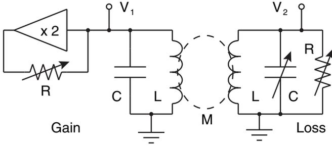
FIG. 1. Electronic implementation of a  $\mathcal{PT}$ -symmetric dimer. The negative resistance gain element is provided by feedback from a voltage-doubling buffer. The coils are inductively coupled, and  $V_1$  and  $V_2$  provide access to the system variables.
