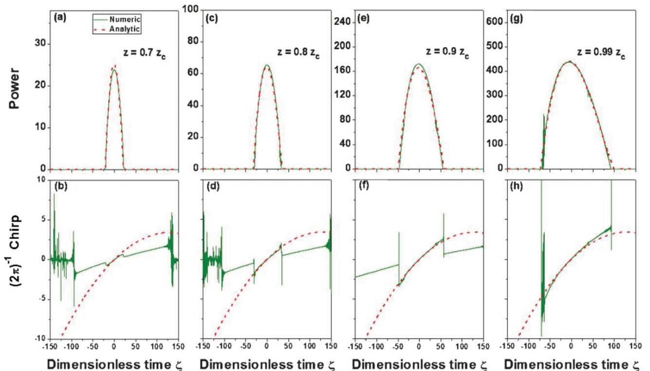
FIG. 7. (Color online) Pulse power profile and chirp of the numerical and analytical renormalized ( $n = 3$ ) solutions for propagating distances  $z = 0.7z_c$  [(a) and (b)],  $z = 0.8z_c$  [(c) and (d)],  $z = 0.9z_c$  [(e) and (f)], and  $z = 0.99z_c$  [(g) and (h)] with  $\mathcal{V}_0 = 3.922 \times 10^{-2}$  and  $\kappa = 3.018 \times 10^{-2}$ .
