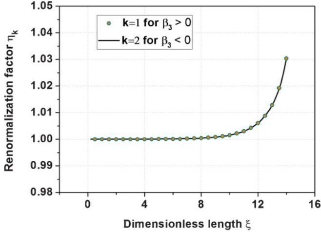
FIG. 2. (Color online) Renormalization functions  $\eta_1(z)$  for  $\beta_3 > 0$  ( $\kappa = 3.018 \times 10^{-2}$ ) and  $\eta_2(z)$  for  $\beta_3 < 0$  ( $\kappa = -3.018 \times 10^{-2}$ ) with input dimensionless energy  $\lambda_0 = 3.922 \times 10^{-2}$ .
