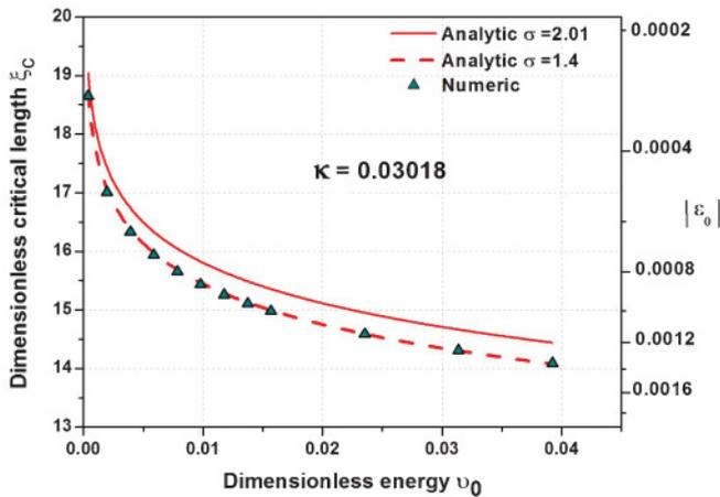
FIG. 9. (Color online) Numerical and analytical (for  $\sigma = 2.01$  and  $\sigma = 1.4$ ) dependence of the dimensionless critical length  $\xi_c = gz_c$  on the dimensionless input pulse energy  $\nu_0$ .
