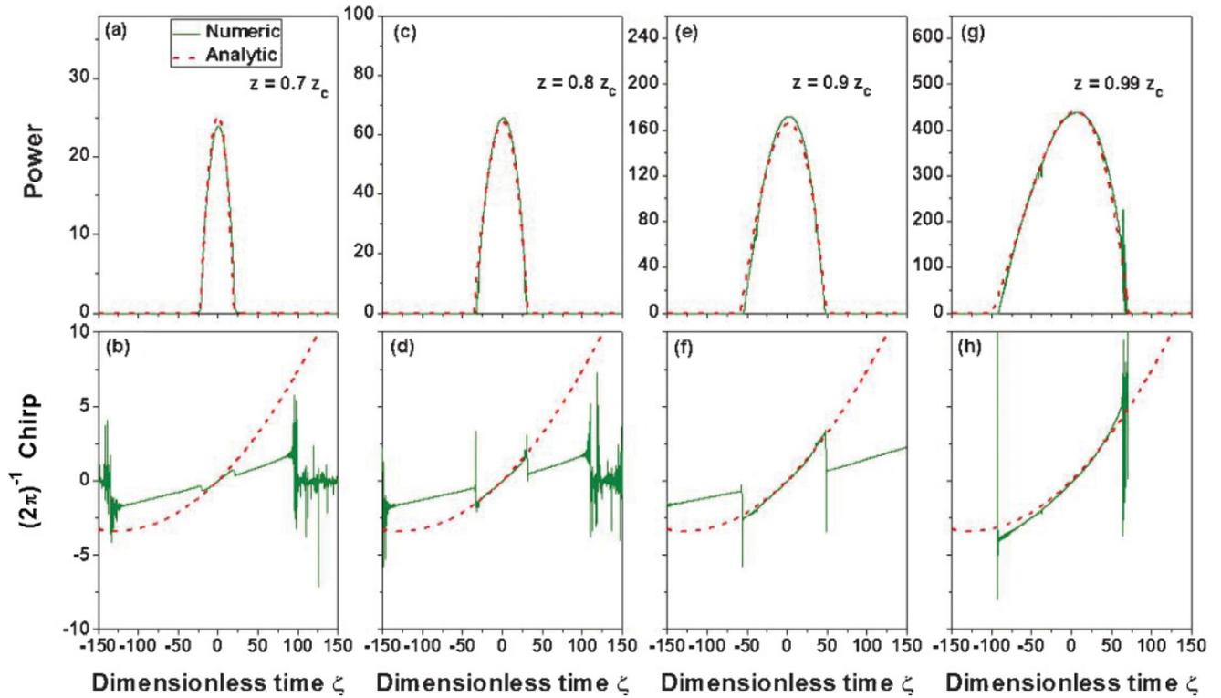
FIG. 8. (Color online) Pulse power profile and chirp of the numerical and analytical renormalized ( $n = 3$ ) solutions for propagating distances  $z = 0.7z_c$  [(a) and (b)],  $z = 0.80z_c$  [(c) and (d)],  $z = 0.90z_c$  [(e) and (f)], and  $z = 0.99z_c$  [(g) and (h)] with  $\nu_0 = 3.922 \times 10^{-2}$  and  $\kappa = -3.018 \times 10^{-2}$ .
