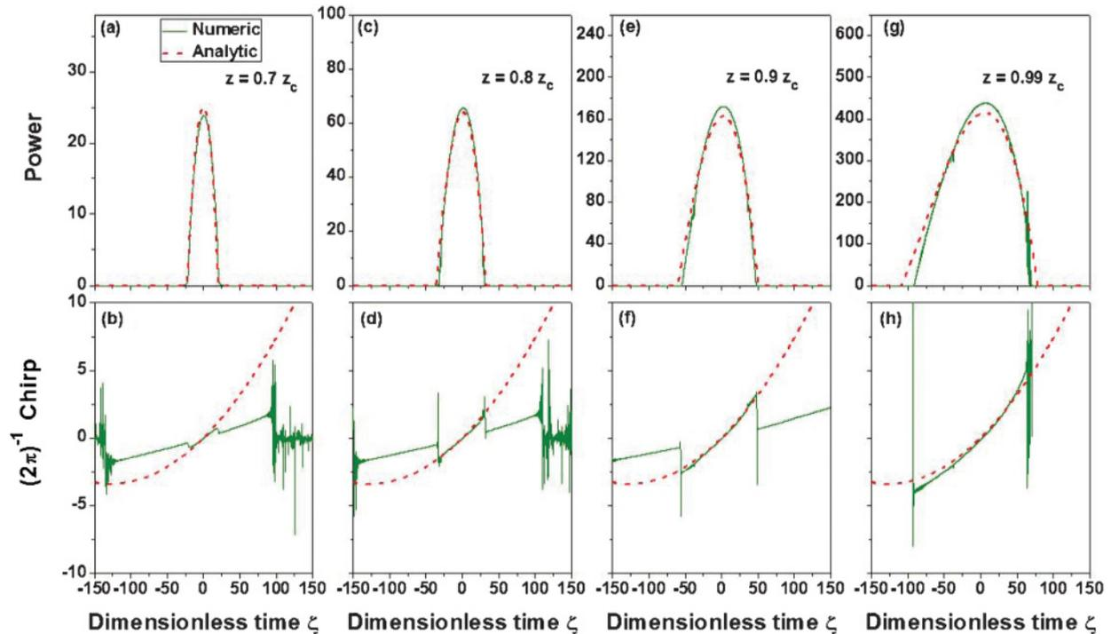
FIG. 6. (Color online) Pulse power profile and chirp of the numerical and analytical (nonrenormalized) solutions for propagating distances  $z = 0.7z_c$  [(a) and (b)],  $z = 0.8z_c$  [(c) and (d)],  $z = 0.9z_c$  [(e) and (f)], and  $z = 0.99z_c$  [(g) and (h)] with  $\mathcal{V}_0 = 3.922 \times 10^{-2}$  and  $\kappa = -3.018 \times 10^{-2}$ .
