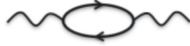
FIG. 16. Lowest-order subdominant Landau-damping contribution to the superfluid stiffness coming from finite fermion density.
