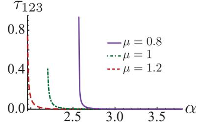
FIG. 4. (Color online) Residual tripartite entanglement in the vibrational state of the transverse modes of our system. We study  $\tau_{123}$  against  $\alpha$  at  $T = 0$  and for three values of  $\mu$ . Each curve is given in a range of parameters such that both stability and the validity of the second-order approach are guaranteed. The residual tripartite entanglement is always finite, with a maximum value that depends on  $\mu$ .
