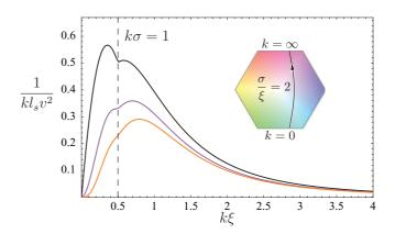
FIG. 5. (Color online) Inverse elastic scattering mean free path, (81), as function of Bogoliubov wave number  $k\xi$  for disorder with fixed correlation parameter  $\zeta = \sigma/\xi = 2$ , in d = 1,2,3 dimensions (top to bottom). For small or large  $k\xi$ , universal limiting behavior is found (see text). The feature at  $k\sigma = 1$  is particular to the speckle disorder [Eq. (A6)]. Inset: the plot's path in the parameter space (Fig. 4).
