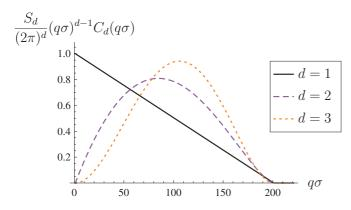
FIG. 11. (Color online) Isotropic speckle correlation function as a function of reduced momentum in d=1,2,3. To show comparable scales, we plot  $[S_d/(2\pi)^d](q\sigma)^{d-1}C_d(q\sigma)$ , including the d-dimensional volume integration element.
