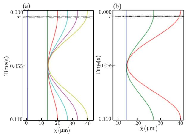
FIG. 3. (Color online) (a) Radio frequencies,  $\omega_n$ , as a function of time to achieve the counterintuitive positioning sequence. (b) Positions of the trap minima as a function of time. The left trap remains stationary while the other two traps move toward it. The delay in the movement of the middle trap in comparison to the right trap ( $\tau = 0.0055$  s) is indicated by the broken line.
