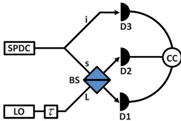
FIG. 2. (Color online) Schematic model of the experiment. The LO photon (L), after a delay  $\tau$ , interfered with the signal (s) at the beam splitter (BS) with the idler (i) as a herald. These photons were detected by three detectors and recorded by a threefold coincidence counter (CC).
