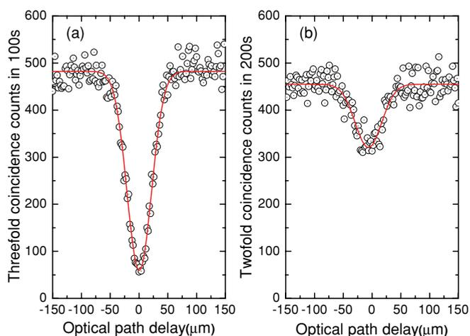
FIG. 5. (Color online) Observed HOM interference. (a) Threefold coincidence counts between the LO and heralded signal, with the idler as the herald. (b) Twofold coincidence counts between the LO and signal, without the herald. No background signals were subtracted in either (a) or (b). The solid curves represent Gaussian fits to the data points.
