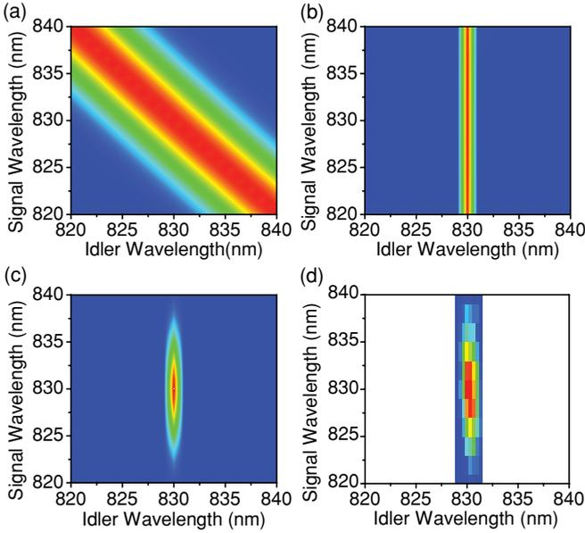
FIG. 1. (Color online) Density plots of the (a) pump-envelope function, (b) phase-matching function, (c) calculated joint spectral distribution function, and (d) experimentally observed joint spectral distribution of the SPDC that we employed.
