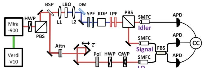
FIG. 4. (Color online) The experiment setup. CC (coincidence counter), APD (avalanche photodiodes), FBS (fiber beam splitter), SMFC (single-mode fiber coupler), PBS (polarizing beam splitter), QWP (quarter-wave plate), HWP (half-wave plate), Pol (polarizer), Attn (attenuator), BSP (beam sampler), DM (dichroic mirror), SPF (short-wave pass filter), and LPF (long-wave pass filter).
