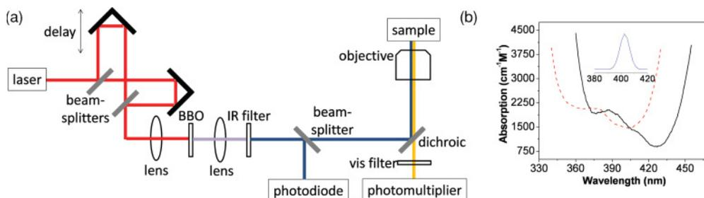
FIG. 1. (Color online) (a) Experimental setup; the scanning mirrors and confocal detection schemes are not shown for simplification. (b) Relevant absorption spectral profiles (lines) of rhodamine-6G in ethanol (solid black) and fluorescein in basic ethanol (dashed red); data were taken from the web resource for spectral database [34] and presented after smoothing over adjacent points. The inset shows the pulse spectra (solid blue).
