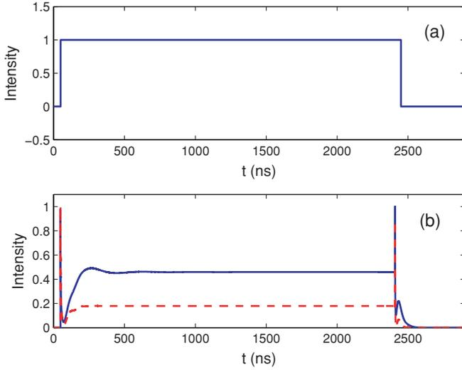
FIG. 2. (Color online) Observation of optical precursors from a square-modulated pulse through a QW system. (a) The input square pulse with no QWs present. (b) The optical precursor signal and delayed main pulse with TIT (blue solid line) and without TIT ( $\kappa = 0$ , red dashed line). Optical depth  $\alpha_0 z \approx 43$  and  $\Omega_c = 0$ .
