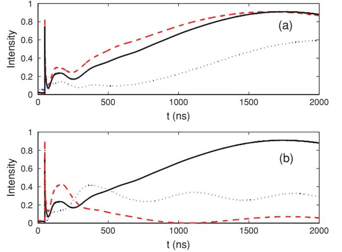
FIG. 5. (Color online) Optical precursor at the rising edge (a) for different optical depths  $\alpha_{0z} \approx 21$  (red dashed curve), 43 (black solid curve), 64 (blue dotted curve) and (b) for  $\Delta_p = 0.72$  meV (red dashed curve),  $\Delta_p = 1$  meV (black solid curve),  $\Delta_p = 1.28$  meV (blue dotted curve),  $\alpha_{0z} \approx 43$ .  $\Omega_c = 0.2$  meV,  $\Delta_c = -0.73$  meV.
